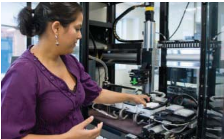
Toxicology at the National Institutes of Health Chemical Genomics Center revolves around assessing compounds using trays with tiny cell-filled wells. Robots can perform thousands of tests in an afternoon. Experiments are conducted at several dosage levels and examine multiple cell effects to ensure precision and accuracy, says Sunita Shukla, a post-doctoral fellow whose position is funded in part through an alternatives award from The HSUS and Procter & Gamble. “We’re not just here to pump out data,” she says. “We’re here to get data that’s meaningful for the toxicology world.”
