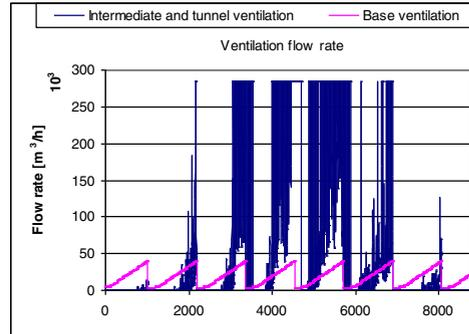
Fig. 4. Base ventilation and tunnel ventilation flow rates
