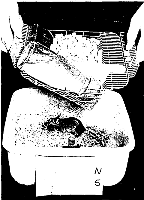
FIGURE 2. The Cambridge cage. The lid is basically a flat expanded wire sheet, bent in three places to form a trough, with a relatively large food compartment separated by a removable divider from the bottle compartment. There is a shelter formed by a solid sheet placed on the shallow slope of the food compartment, and the area under the food compartment is low enough (2.2 cm) at the ridge so that the nest area under the shelter can be made "snug." It fits onto a shallow smooth-rimmed plastic bowl. The overall internal dimensions of the bowl are: 27 cm x 22 cm x 8 cm (height); volume, 4,750 cc.
